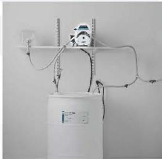
11) Close valve 4. 12) To dispense- Open valves 3 and 7. Run pump only when dispensing.
