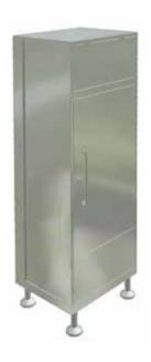
This cabinet is designed to assist in the degowning and collection of soiled garments for washing. The top flap allows for easy disposal and the door has a latch allowing easy emptying by cleaning contractor. Fabrication material stainless steel 304 electropolished finish.
