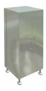
Cleanroom Full Length storage cabinets with 2 swing doors. All shelves are removable. Available with either leveller legs or on casters. Sloping roof is standard. Fabrication material stainless steel 304 with electropolished finish.
